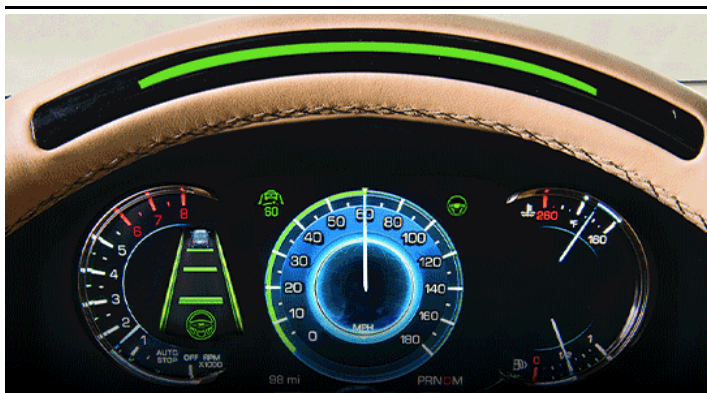
Figure 20: First Alert (steering wheel flashes green)
