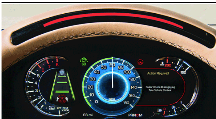
Figure 21: Second Alert (steering wheel flashes red)
