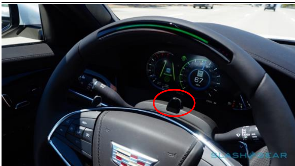
Figure 19: GM Cadillac CT6 with Super Cruise (note camera circled in red)
